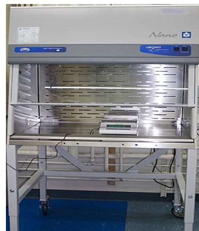
Example of HEPA-filtered hood at UCSB specifically for nanomaterial use
