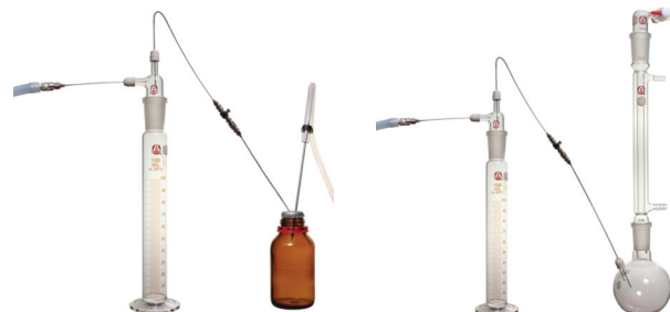
Fig. 12 Double-tipped needle transfer to graduated cylinder
