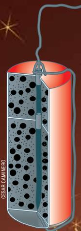
**Figure 1. Structure of an aerial shell. The black balls are the stars, and the gray area is gunpowder. The stars and the powder are surrounding a bursting charge, which also contains black powder.**
